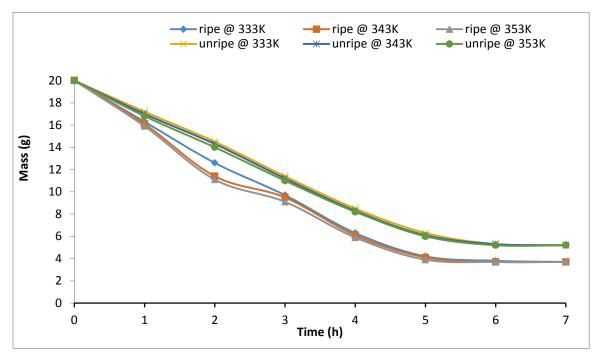
Figure 4 Mass (g) of the plantain sample against time (h) at various regulated drying temperatures
