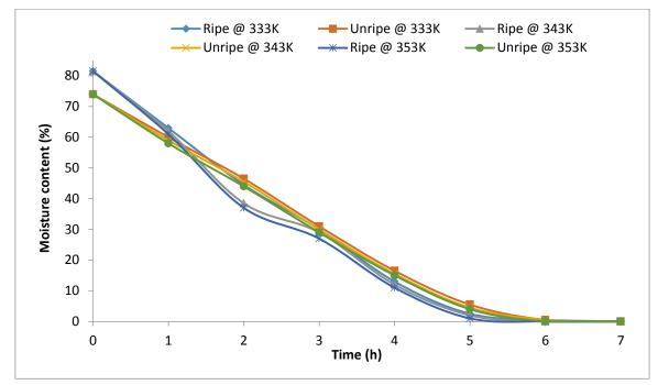
Figure 5. Percentage moisture content (%) against time (h) of the plantain samples at various regulated drying temperatures
