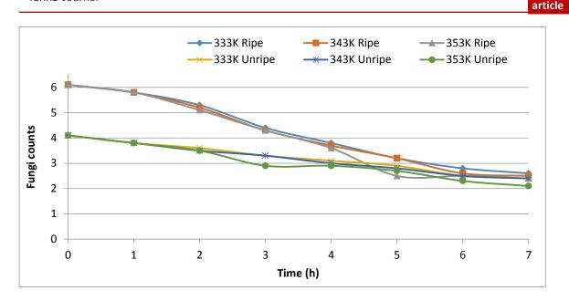
Figure 8 Fungi counts of the plantain samples against time (h) at various regulated drying temperatures.
