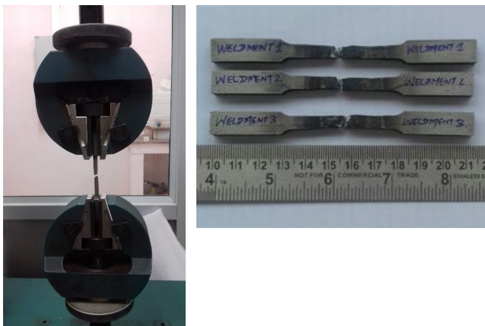
Figure 3: Universal testing machine set up (b) Sample loaded in machine (c) Room temperature samples
